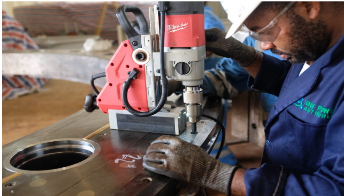
Figure 8: Drilling thread holes on the repaired bottom ring surface
